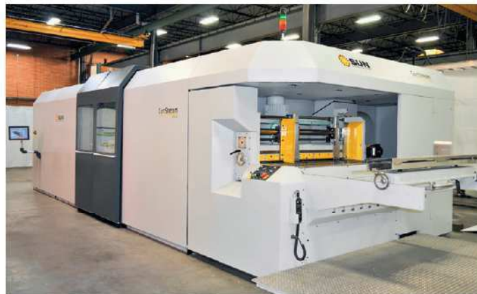
Sun Automation's Corr-Stream machine prints CMYK with water-based inks
